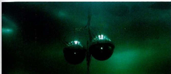
Top: the central trigger electronics in its pressure glass spheres, ready to descend into Lake Baikal. Bottom: a pair of light sensors in water about 10 m below the ice cover of the lake, before deployment to a depth of 1.1 km.
