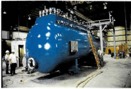
Coldbox in final stage of fabrication at the Linde shop in the Port of Catoosa, Oklahoma, USA
